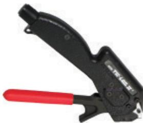
For applying 4.5mm wide smooth ID Mini Tie-Lok® ties for cable bundling and identification tagging. Forms unique dimple lock with a strong locking force and cuts off the excess band flush with top of buckle so the completed lock is smooth and not sharp.
