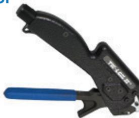
Applies 6.35mm wide smooth ID Tie-Lok® ties used in cable bundling and identification tagging. Locks tie with the patented Tie-Lok® and cuts off excess band flush with top of buckle so the completed lock is smooth and not sharp.
